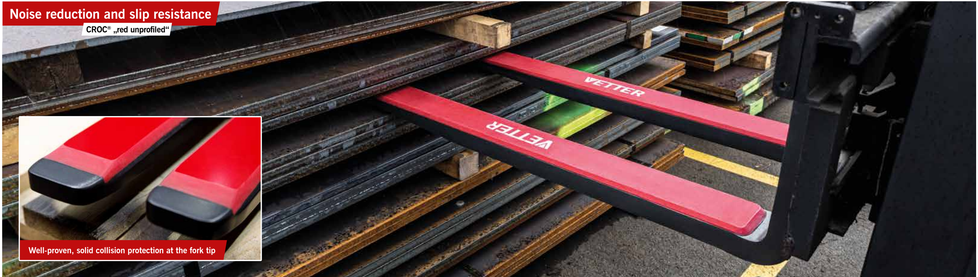
CROC® coating „red“: noise reduction when transporting steel plates
